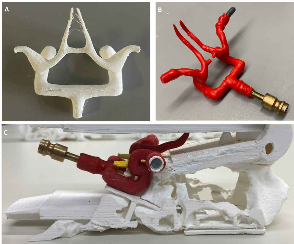
Figure 21: A) Hollowed-out 3D printed model of the CAW B) latex-based CAW model (earlier version) C) finished CAW model coated with latex and embedded in the central console with magnetic adapters attached on both proximal M1 segments.
