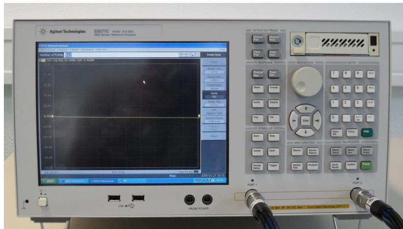
Figure 6.3: The Network Analyzer (Agilent ENA E5071C).
