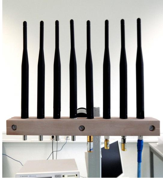
Figure 4.3: The designed ULA composing 8 elements.
