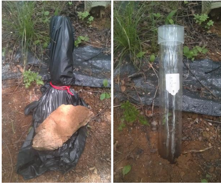
Figure S2. Photographs of one minirhizotron installed in BEF China with a plastic cover (left) and unsealed (right).
