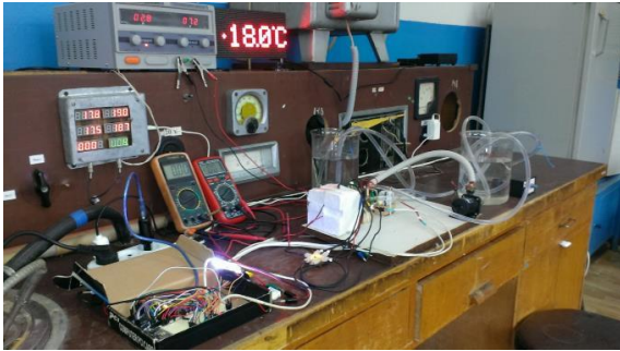
Figure 3: Workplace for the study of a thermal power generator.
