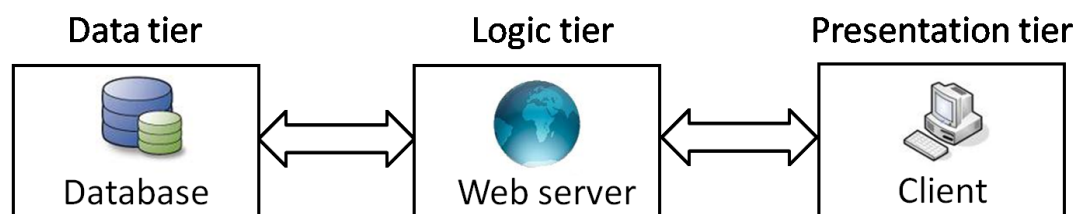
Figure 1: The three-tier architecture is being instantiated by the DBE2 information system. The presentation tier (the DBE2 client ) calls the logic tier to download, upload, and edit biological data. The logic tier (the DBE2 servlet ) employs the data tier (the DBE2 database and a file storage system) for the storage of experiment data and binary files. This happens using an underlying user management to manipulate or transfer data by defined queries.
