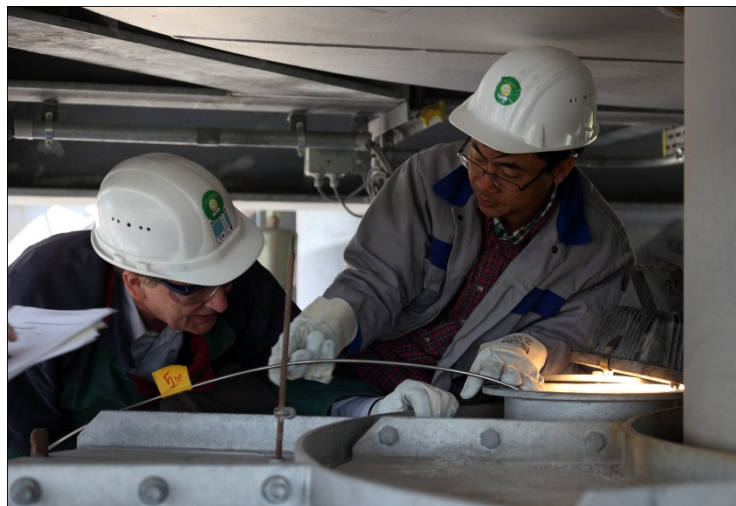
Figure 7-3: Inserting thermocouples during measurements
