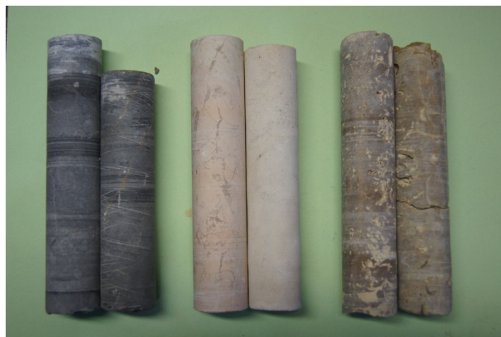
Figure 3-5: Cylindrical samples of limestones from different sources
