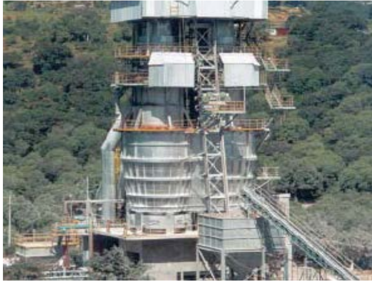
Figure 1-7: PFR- kiln (source: http:// www.maerz.com )
