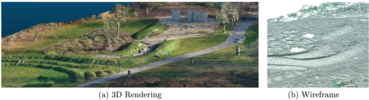
Figure 11.3: Calculated SFM 3D model of the playground (from [Bolten et al., 2022b]).
