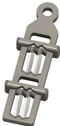
Fig. 2. Custom designed substrate holder made from polylactide for polyelectrolyte immersion of glass scaffolds.
