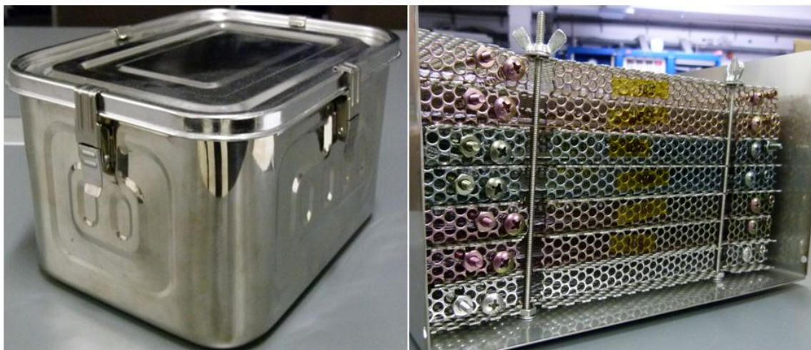
Figure 64: Transport system for coated single fibers consists of stainless steel box (left picture) and the stainless steel brackets (right picture)
