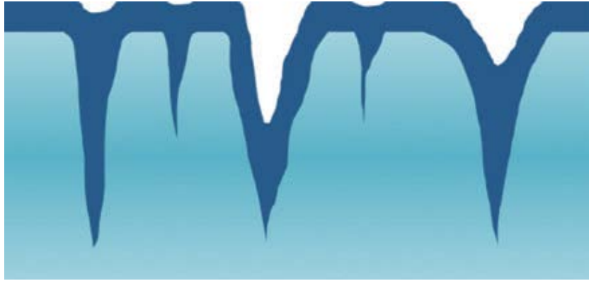
Figure 25: Schematic illustration of ALD coated glass, the surface of glass (bright region) is covered by nanoscale defects, ALD coating (dark region) fills the cracks completely or partially [136]
