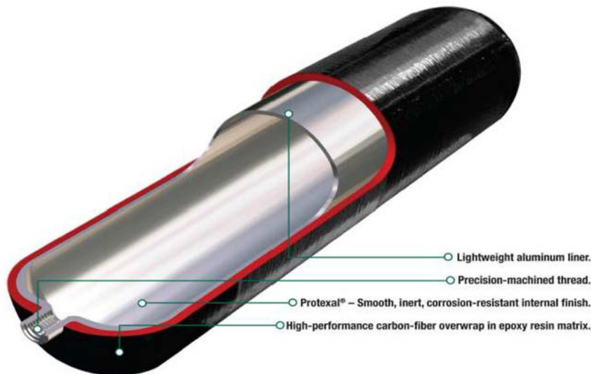
Figure 1: Gas cylinder type III with aluminum liner and carbon fiber wrap [19]
