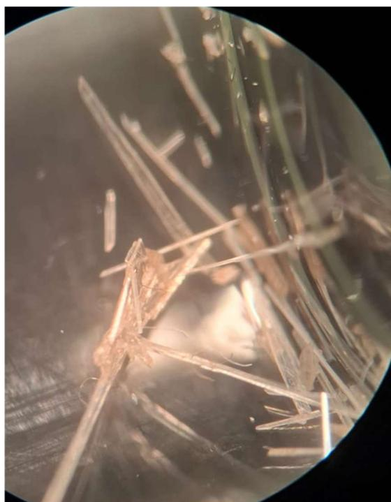
Figure 13: Crystals obtained in the presence of 4-FBN under the microscope
