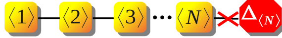
Figure 4.3: Illustration of an EV hierarchy. The black lines indicate the linear coupling between the EV of increasing order. One can imagine the hierarchy as a line of EVs coupled by linear differential equations to the next order. The hierarchy is truncated by setting the (N + 1) EV to zero, i.e. applying the truncation operator \Delta_{\langle N \rangle} .
