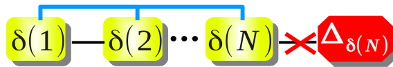
Figure 4.4: Illustration of a CF hierarchy. The CF of a certain order couple linearly to the CF of the next order indicated by the black line, but also to products of lower-order CF indicated by the blue merging lines on top. To truncate the hierarchy at order N the (N + 1) th CF is set to zero i.e. the truncation operator \Delta_{\delta(N)} is applied. In contrast to the EV hierarchy depicted in Fig. 4.3 the CF hierarchy cannot be imagined as a straight line, due to the nonlinear coupling of the CF. The structure of this hierarchy is nonlinear and has to be imagined as an intertwined chain.
