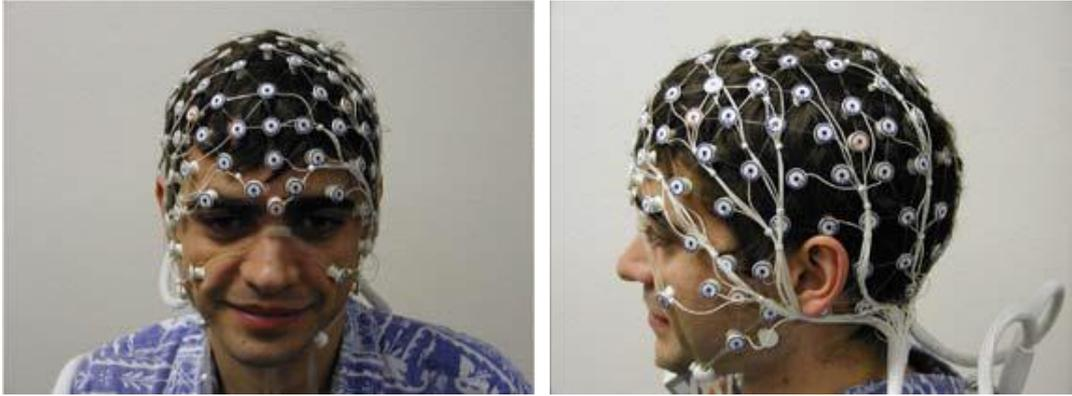
**Fig.9.** EGI 128-channel HCGSN, front (left) and side (right) views.
