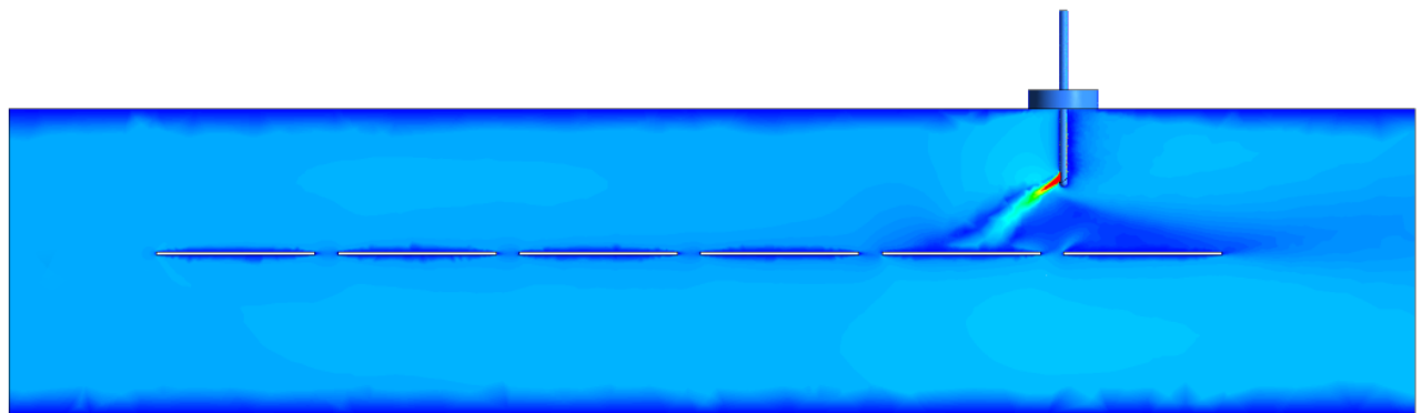
(ii) Second model (air suction by bore hole in the roof insulation)
