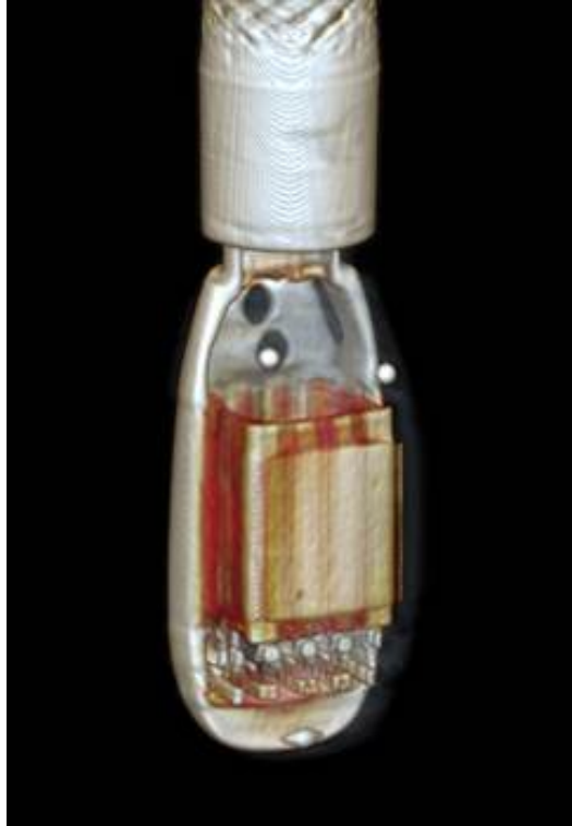
Figure 4.5: Volume rendering of the Mirco-CT of the TEE probe.
