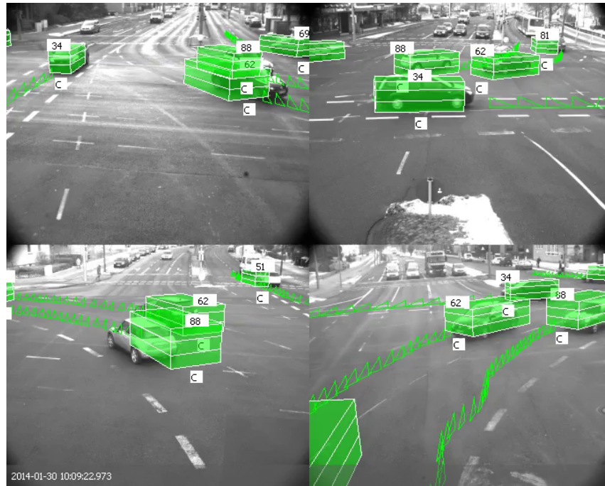
Figure 6.4: Screenshot of the video data used for calibrating the parameters of the car-following model. The green boxes indicate identified objects, green triangles visualize their predicted movement.
