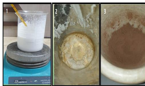
Figure 2. Steps for preparing MoS 2 nanoparticles by sol-gel method
