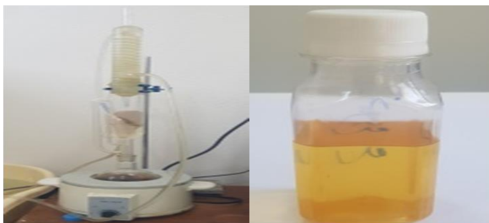
Figure 4: Steps for preparing orange peel extract using the Soxhlet device.
