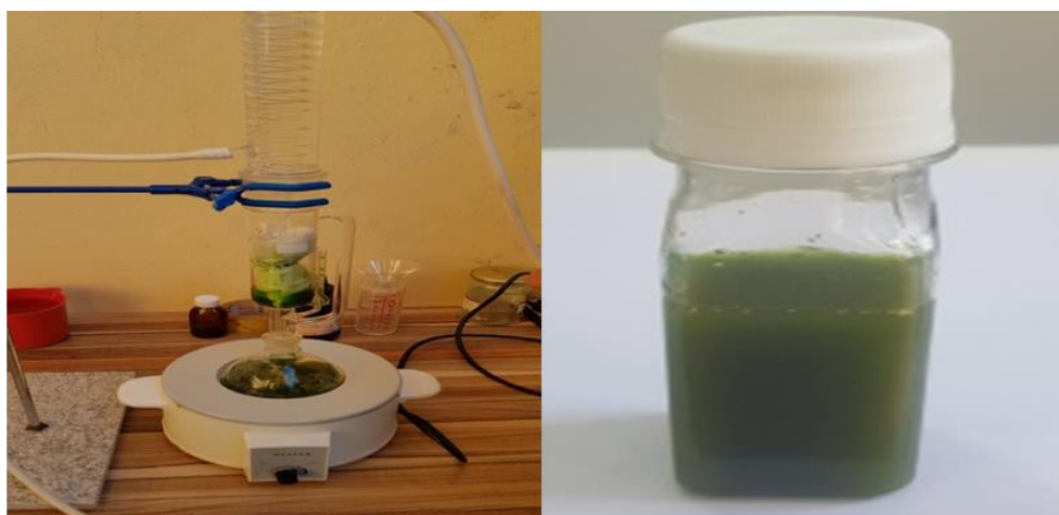
Figure 3: Steps for extracting thuja leaves using a Soxhlet.
