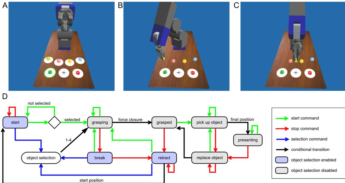
Figure 4.1: Virtual scenario showing the robotic gripper in the states *start* (A), *grasped* (B) and *presenting* (C) and the state diagram (D). The figure originally has been published in [173].
