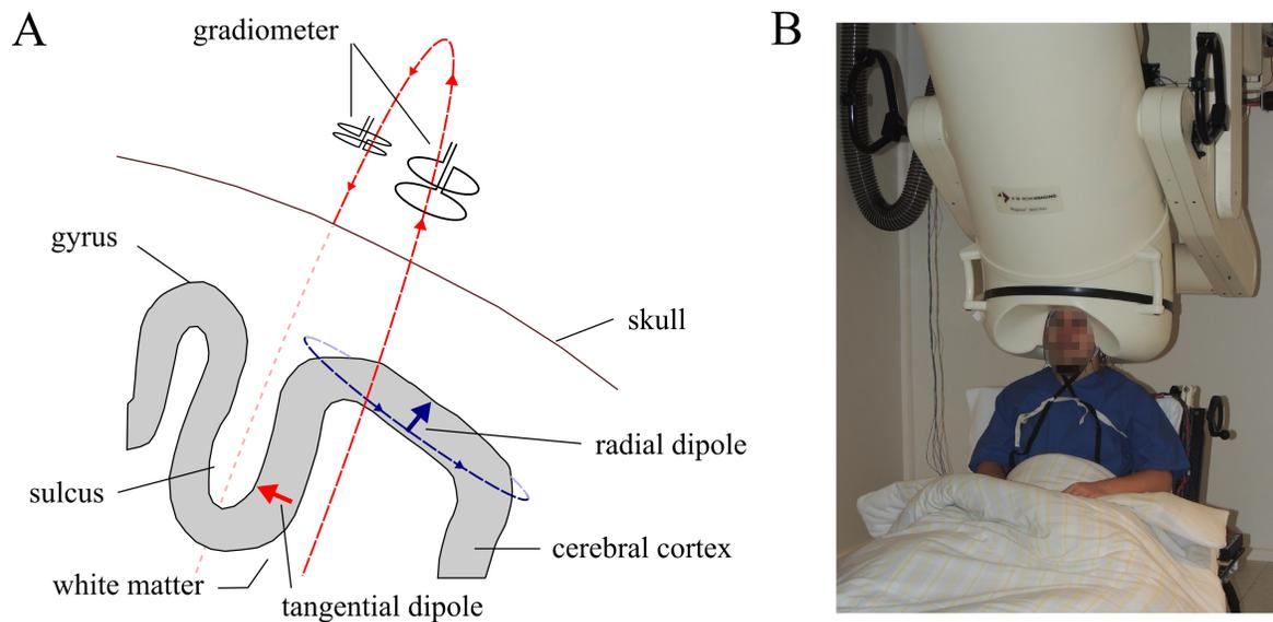
Figure 2.5: Principle of MEG measurement (A). MEG Dewar positioned over a subject (B).
