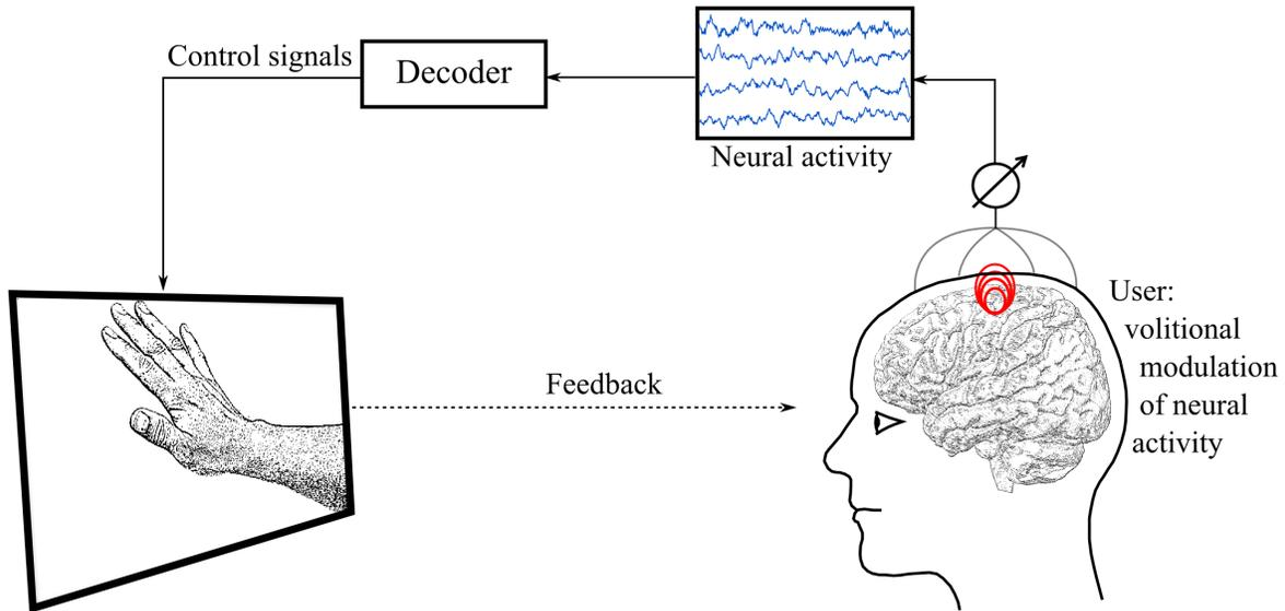
Figure 3.1: Schematic demonstration of a BCI's closed-loop.
