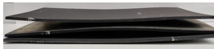
Figure 2.5: Aluminum alloy AA6082 deformed plates
