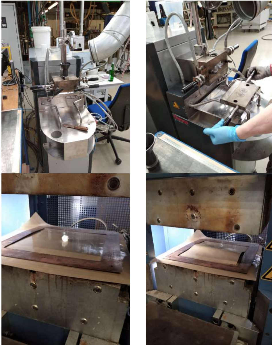
Figure 6: The top images show the kneader with the fabricated polymer melt after the kneading process. The pressing process is exemplary displayed in the bottom pictures.
