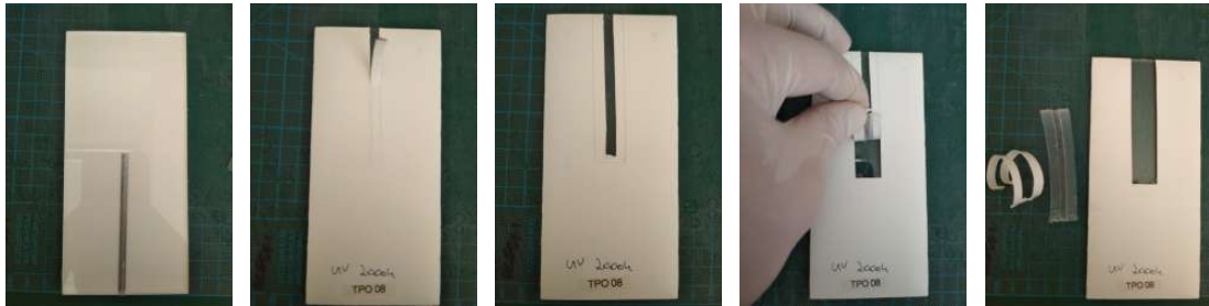
Figure 1. Sample preparation (from left to right) of the weathered coupons.
