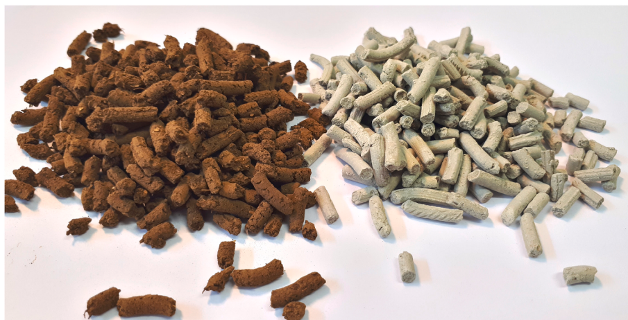
Fig. 1. Manufactured Fe-sludge pellets (left) and clay mineral pellets (right).
