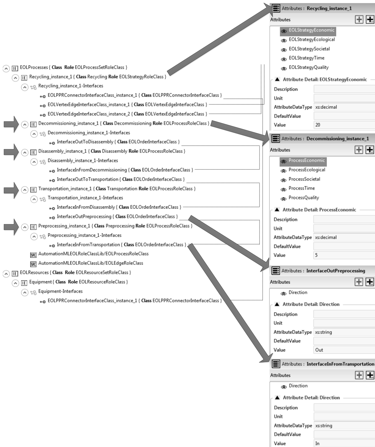
Figure 6.34: Process chain of the End-of-Life strategy 'Recycling' (excerpt)
