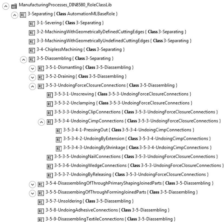
Figure 6.19: DIN 8591 (disassembly processes) as AutomationML role classes
