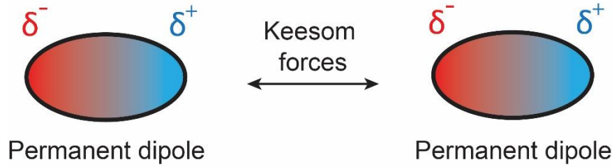
Figure 3: Schematic of Keesom forces. Keesom forces exist between two freely rotating permanent dipoles.
