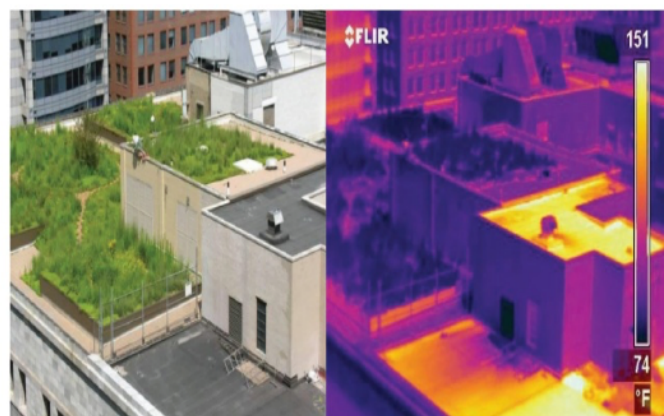
Figure 101- Shows the heat on green and conventional roofs.
