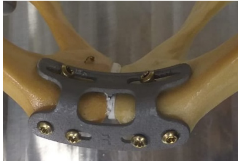
Figure 1. Top view of a specimen with the NSP for self-aligning pubic symphyseal osteosynthesis. The moment one side of the implant is attached, the other pelvic hemisphere can be gently pressed against the predetermined structure of the implant, thereby self-aligning both hemispheres vertically and horizontally.
