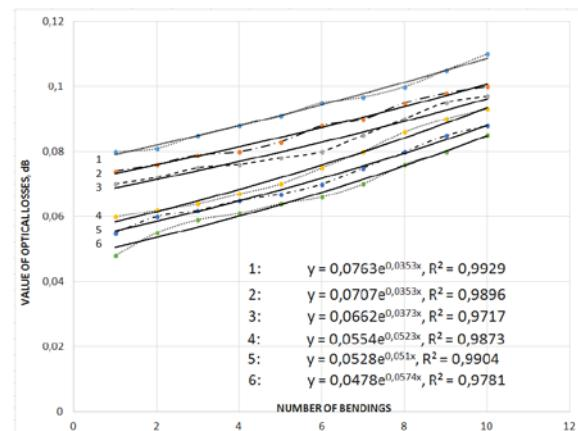
Figure 2: The value of the optical losses of SNR-UT-12 fiber optic cable. The value of the radius r for the curves: 1: 3 mm, 2: 5 mm, 3: 10 mm, 4: 12 mm, 5: 15 mm, 6: 18 mm.
