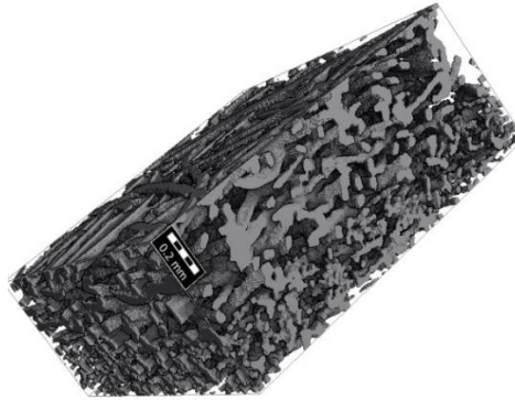
Figure A-2: Micro-CT scan of the domain used for porosity and permeability calculations.
