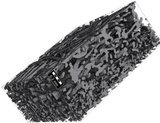
Figure 1-3: A PTL with two different fiber diameters ( 25 \mu\text{m} and 40 \mu\text{m} ) manufactured by Sylatech GmbH, Germany. This PTL has thinner fibers (also smaller pore sizes) towards the CL intended for a better contact with CCM and larger pores towards the water inlet.
