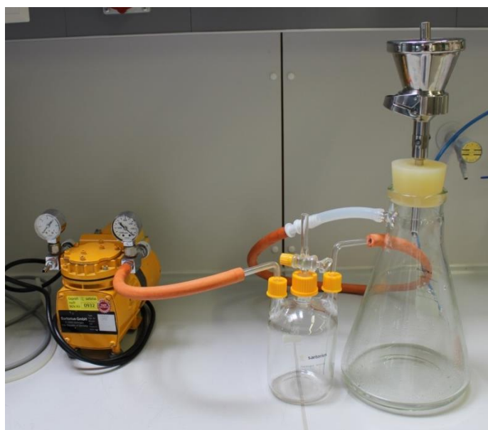
Figure 54: Multi-use büchner funnel with a polyethersulfone-(PESU)-membrane (0.2 µm), plugged to a vaccum pump for the separation of \text{MnO}_2 .
