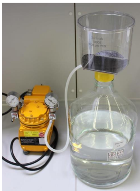
Figure 53: Single-use büchner funnel (180C6, 0.22 µm PES), plugged to a vaccum pump for the separation of \text{MnO}_2 .
