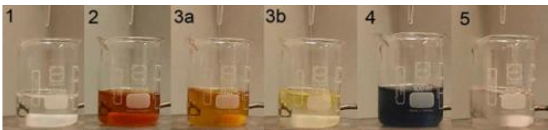
Figure 5: Colour changes during the measurement of the H_2O_2 concentration. From left to right: 1. Acidified KI-solution before the addition of the H_2O_2 sample / 2. Acidified KI-solution after the addition of the H_2O_2 sample / 3a. and 3b. Titration of Na_2S_2O_3 / 4. Addition of the starch solution / 5. End point of the titration.
