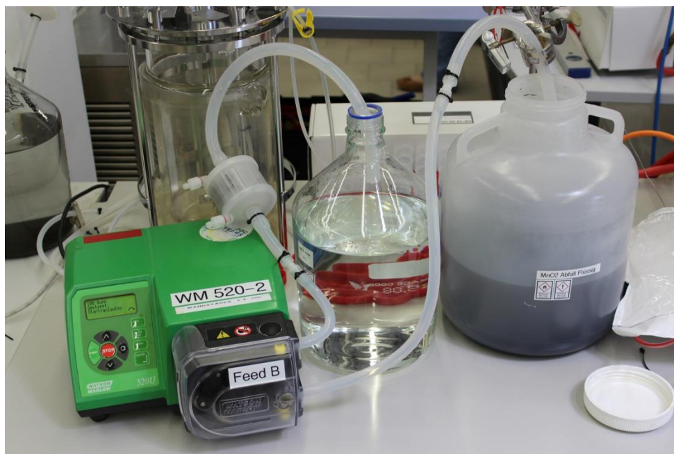
Figure 55: Filtration capsule (Sartopore 2 (0.45 \mu\text{m} + 0.2 \mu\text{m} )), plugged to a peristaltic pump for the separation of \text{MnO}_2 .
