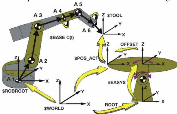
Fig. 3. Robot with external axes and extended kinematic system
