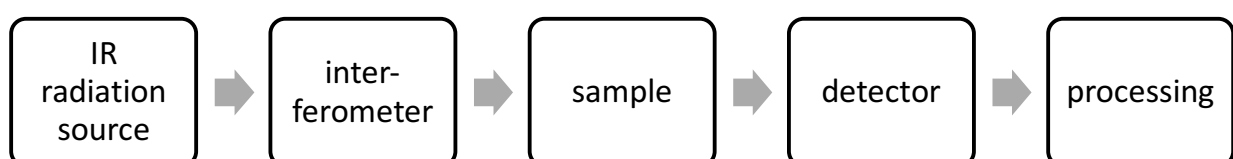
Figure 7: Block diagram of an FTIR spectrometer
