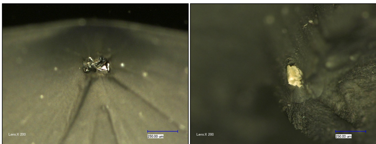
Figure 26: Fractured surface of PP2 contaminated tensile bars
