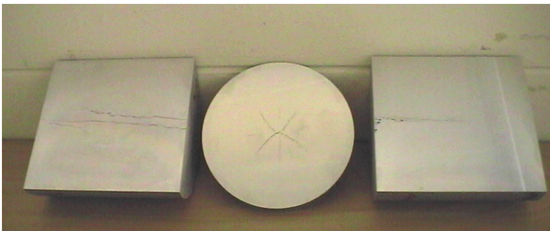
Figure 1.5: General hot cracking pattern observed in Al-Cu billet cast [5]
