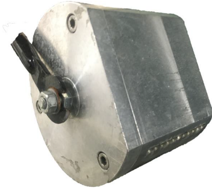
Figure 3.1: Mold with array of 11 jets replicating the secondary cooling
