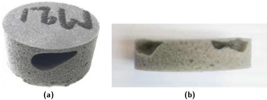
**Figure 4.6:** Examples of non-uniformly distributed random size bubbles inside the foam samples resulting from the manufacturing process.
