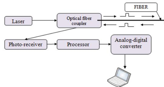
Figure 1: Structural diagram of the system developed.
