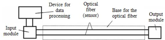
Figure 3: Structural diagram of the method based on the use of micro-stresses of mechanical action on the optical fiber.
