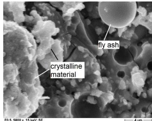
b) F05 showing crystalline material and a fly ash sphere
