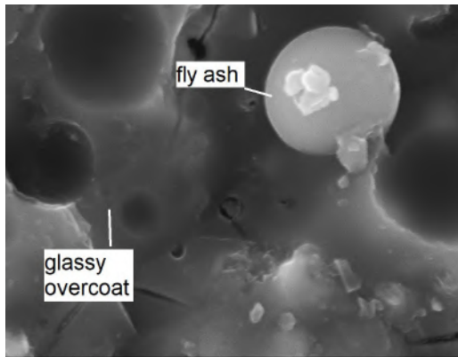
e) F08 showing a glassy overcoat over the sample and fly ash spheres
