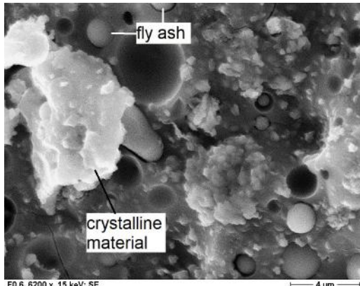
c) F06 showing small fly ash spheres and growing crystalline material
