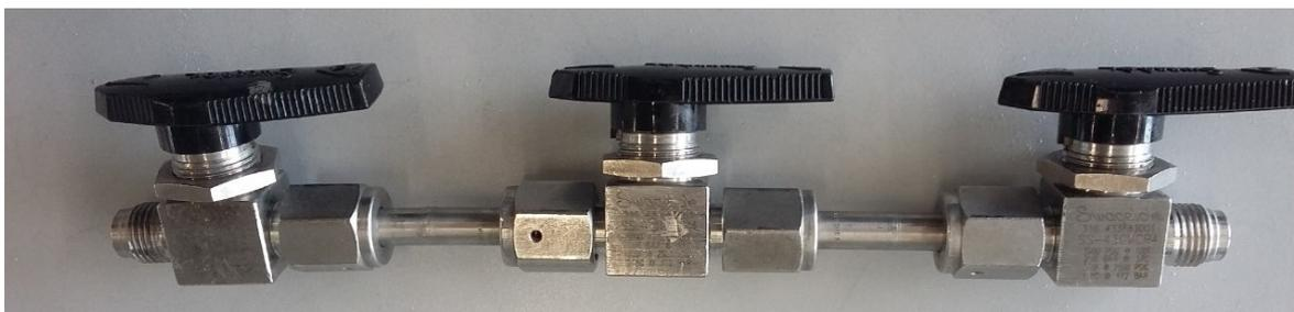
Figure 22: Injection feeder
