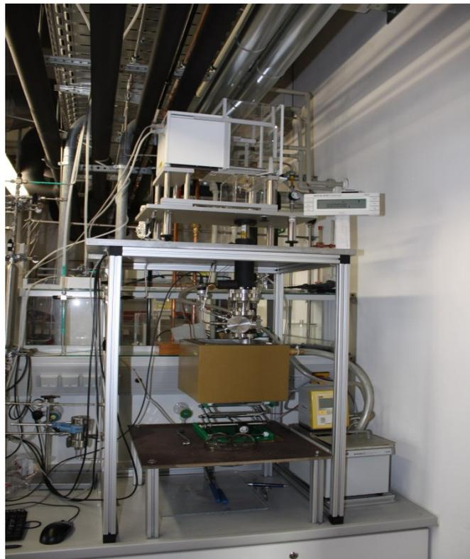
Figure 28: High pressure sorption balance
