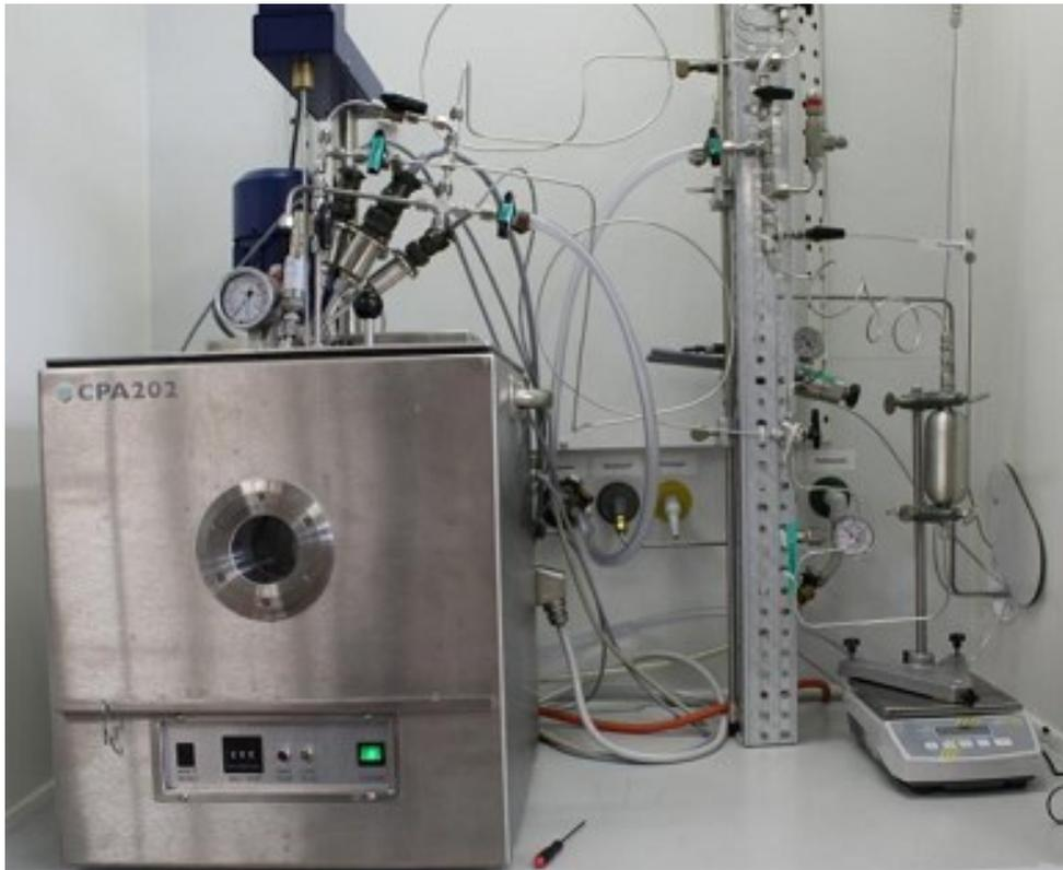
Figure 17: 0,25-liter reactor set-up
