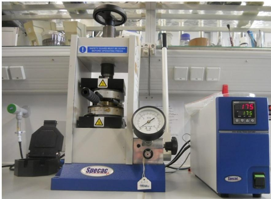
Figure 32: Powder press for film fabrication
