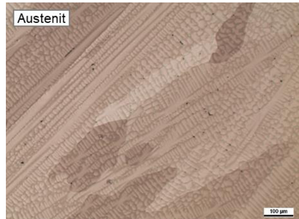
b) \phi_{\text{HC340LA}} = 10\% , 0 FN, 194 HV10, V: 100x
