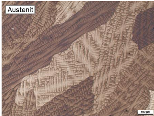
a) \phi_{\text{HC340LA}} = 0\% , 0 FN, 199 HV10, V: 100x
