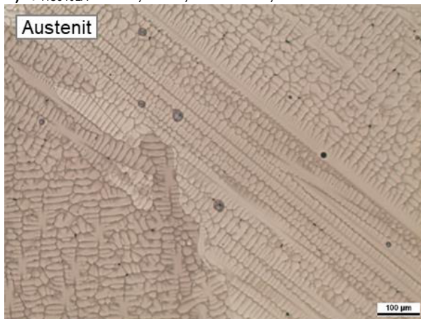
c) \phi_{\text{HC340LA}} = 20\% , 0,1 FN, 196 HV10, V: 100x
