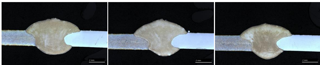
Figure 60: Influence of the sampling position on seam geometry and dilution using the example of a lap weld of the material combination of FeMn-II (upper sheet) + 22MnB5+AS150 PH (lower sheet) + FM-I. Etching: Klemm I
