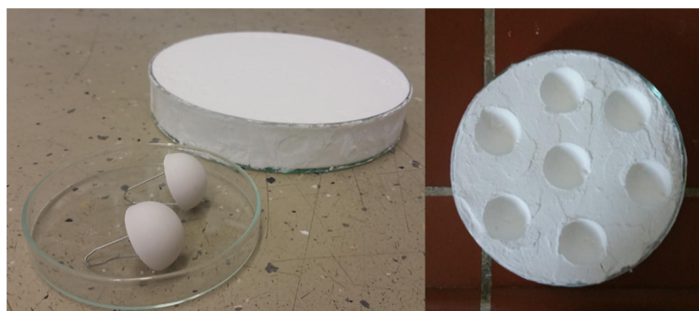
Figure 4.2-4: Shaping technique (left:Stamps and powder tray, right: Molds)
