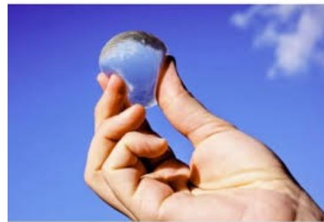
Figure 2.2-3: Small edible water bottle made by alginate [Ooh17]
