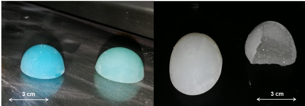
Figure 5.9-4: Crystalline containers with addition of color (left) and flavor (right) [Wel18c]
