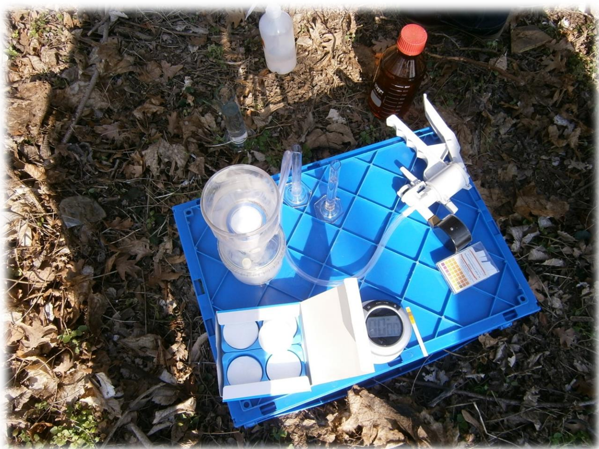
Figure 4-24: Complete equipment for field sampling using developed selective filter-paper disks
