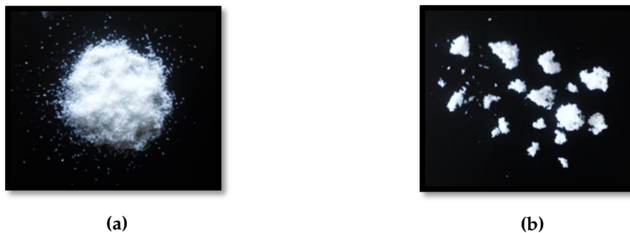
Figure 2.2: (a) Maltodextrin primary particles and (b) agglomerates produced in spray fluidized bed.
