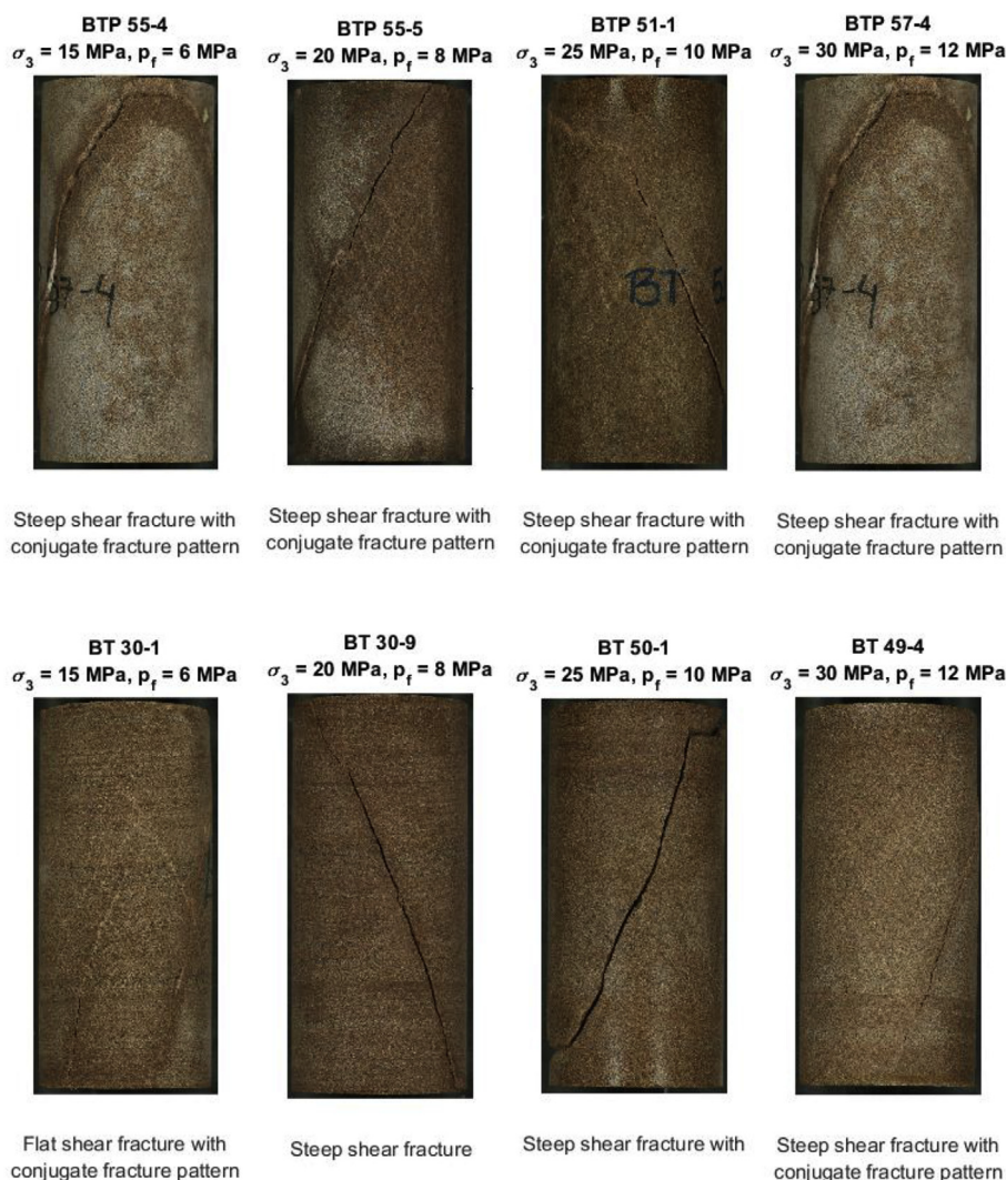
Fig. 13. Fracture pattern of Rotliegend core specimens drilled either parallel (upper row) or transverse (lower row) to bedding. The samples correspond to the deformation tests from Fig. 11a and b. Pictures taken with a core sample scanner.
