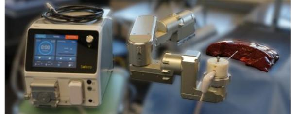
Figure 1: Interventional robotic platform consisting of an ablation and a surgical robotic device, moving the needle through the specimen.
