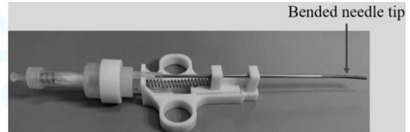
Figure 2: Biopsy device with bended NiTi needle tip.
