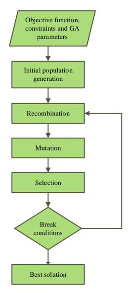
Figure 4.1 Flowchart of the genetic algorithm
