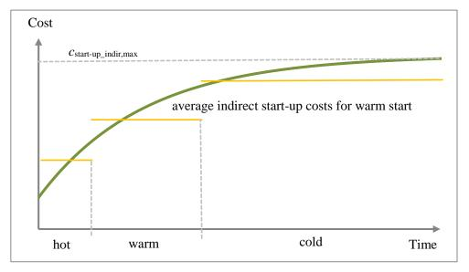
Figure 3.9 Indirect start-up cost function [41]
