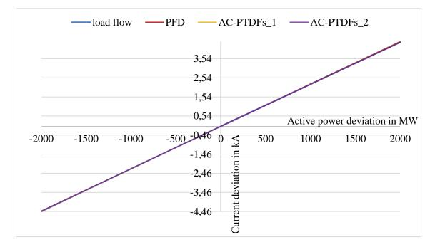
Figure 3.5 I-P characteristics for the line 'L3' in the '5 Bus' IEEE test network model
