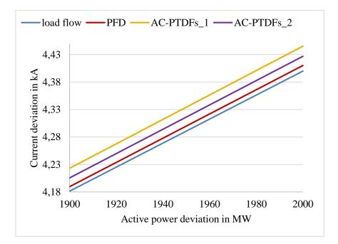
Figure 3.6 I-P characteristics for the line 'L3' in the '5 Bus' IEEE test network model (zoomed representation)
