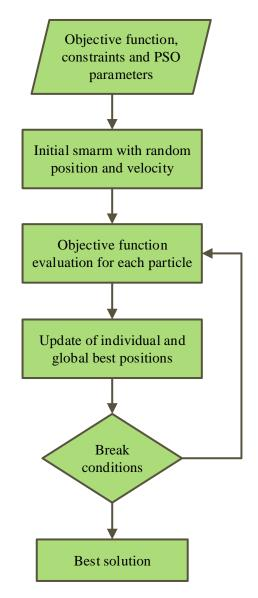
Figure 4.5 Flowchart of particle swarm optimization
