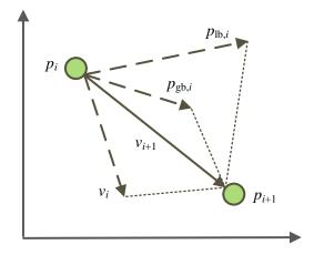
Figure 4.4 Particle movement
