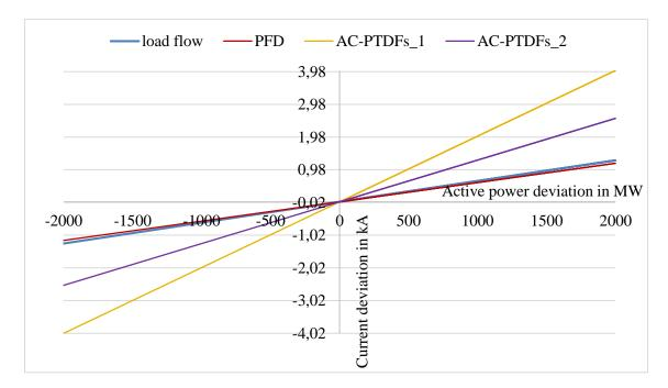
Figure 3.7 I-P characteristics for the line power line between bus bars '1' and '2'
