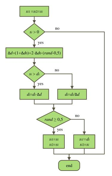
Figure 4.3 Algorithm for the determination of the shape variables
