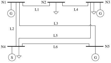
Figure 3.2 '5 Bus' IEEE power grid model
