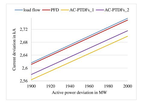
Figure 3.4 I-P characteristics for the line 'L1' in the '5 Bus' IEEE test network model (zoomed representation)
