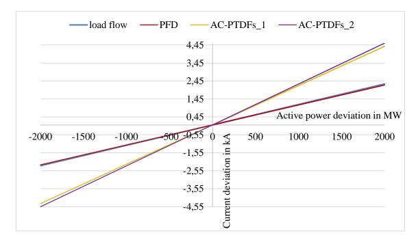
Figure 3.8 I-P characteristics for the line power line between bus bars '11' and '19'
