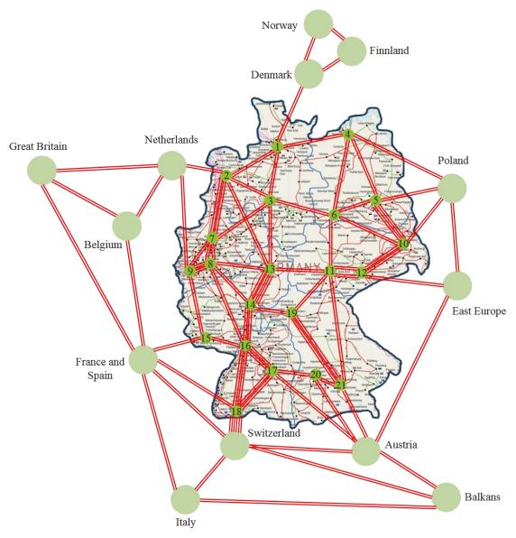
Figure 5.3 Simplified ENTSO-E network model [98]
