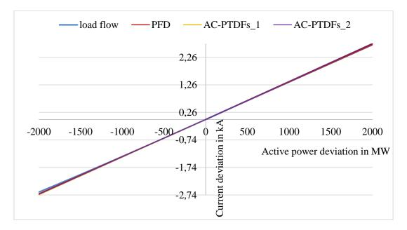
Figure 3.3 I-P characteristics for the line 'L1' in the '5 Bus' IEEE test network model
