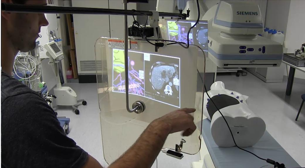
Figure 5.7: Projector and LMC mounted onto the radiation shield with a custom 3D-printed mount.
