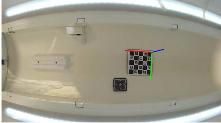
Figure 4.10: Estimation of the fixed ChArUco marker pose for registration of the MRI coordinate system with the camera coordinate system. ©2018 John Wiley and Sons
