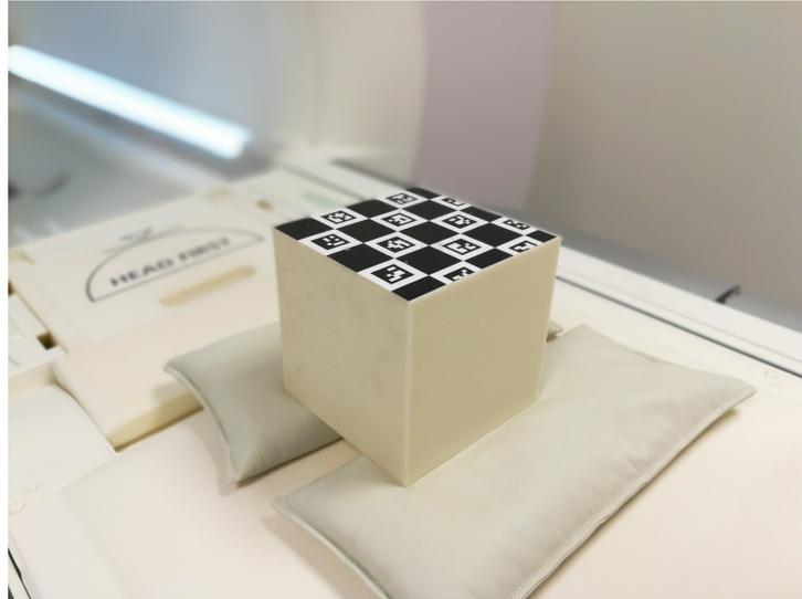
Figure 4.11: Calibration body filled with candle wax for MRI imaging and with a ChArUco board attached to estimate the phantoms pose in camera coordinates. ©2018 John Wiley and Sons
