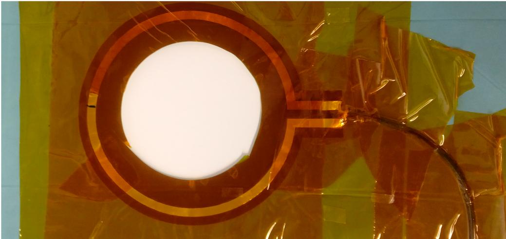
Figure 4.20: A flexible MRI coil integrated in a sterile drape for interventional use [222].
