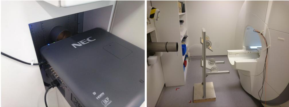
(a) Projector outside the scanner room in (b) The mirror stand and waveguide on the front of the waveguide. MRI's head side.
