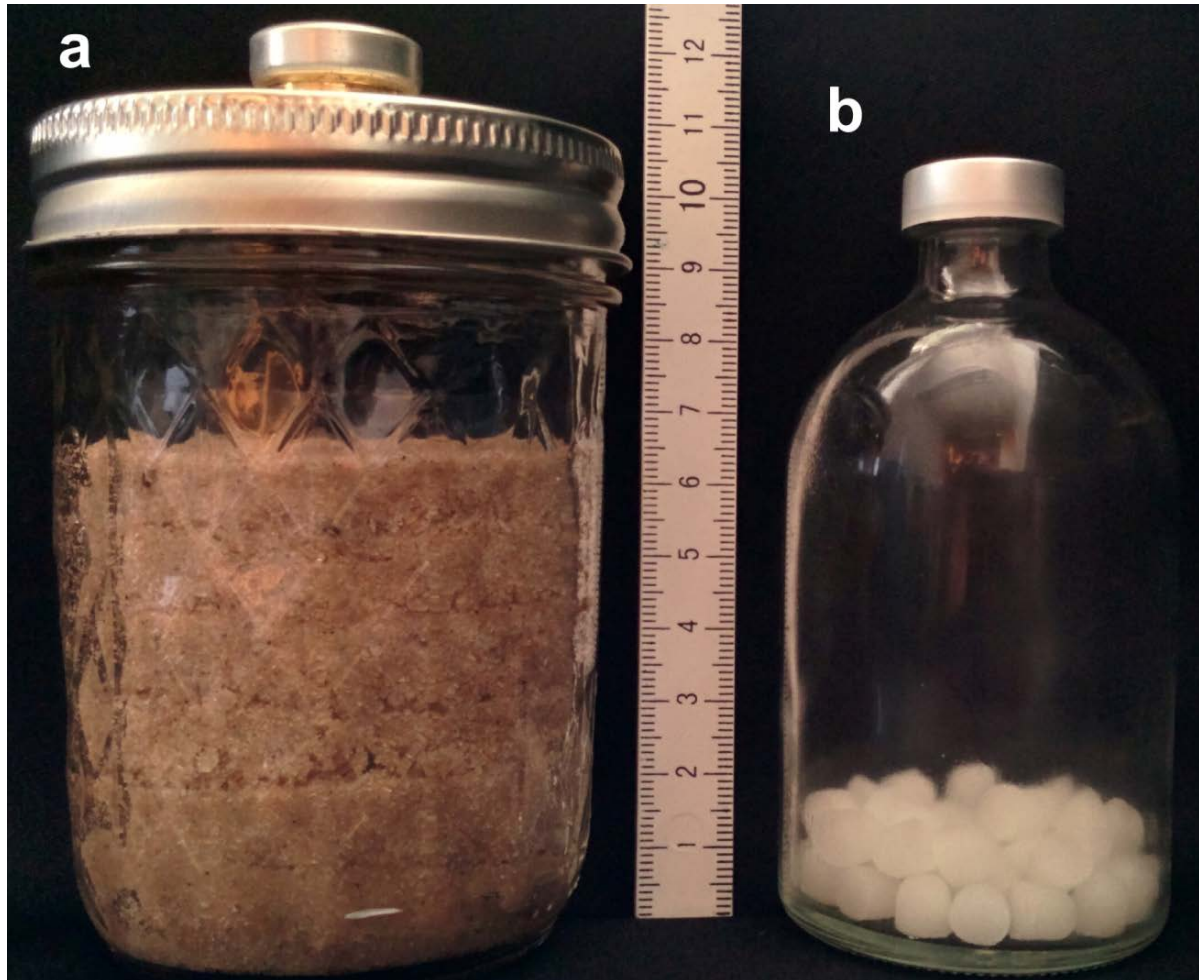
Figure S 8: (a) Half-pint incubation jar (230ml) filled with sand and porous glass beads that serve as microbial hotspots. (b) Respiration kinetics of different types of hotspots either inoculated with Agrobacterium tumefaciens or Paracoccus denitrificans are measured with 50 hotspots in an otherwise empty glass jar (120ml). Note that hotspots are packed densely with minimal distance, which might have affected aeration.
