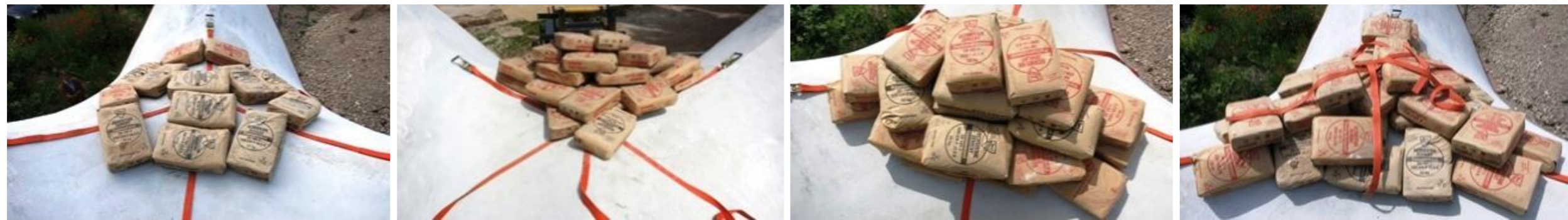
Load Test I-1 – 13 bags ~ 325 kg. Load Test I-2 – 20 bags ~ 500 kg. Load Test I-3 – 30 bags ~ 750 kg. Load Test I-4 – 33 bags ~ 825 kg.
