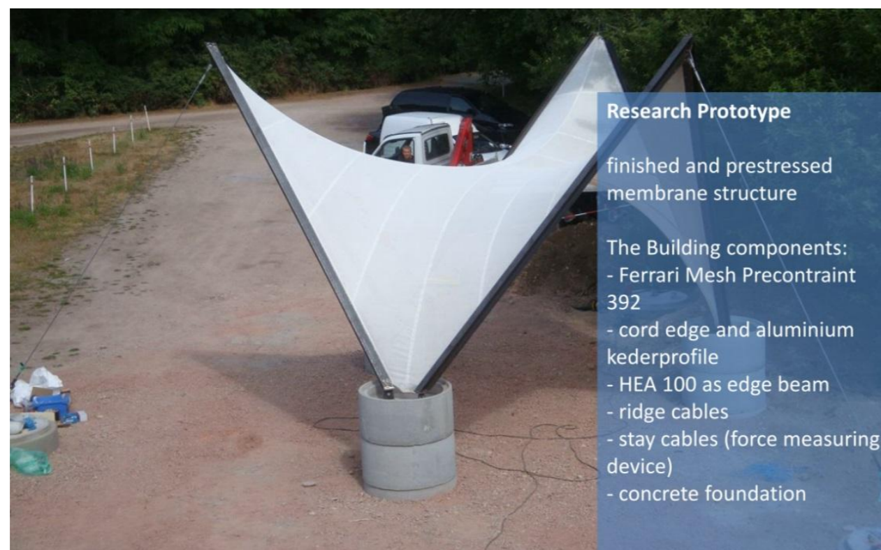
a) Prototype with Tensioned Membrane, Steel, Cables, and Footings
