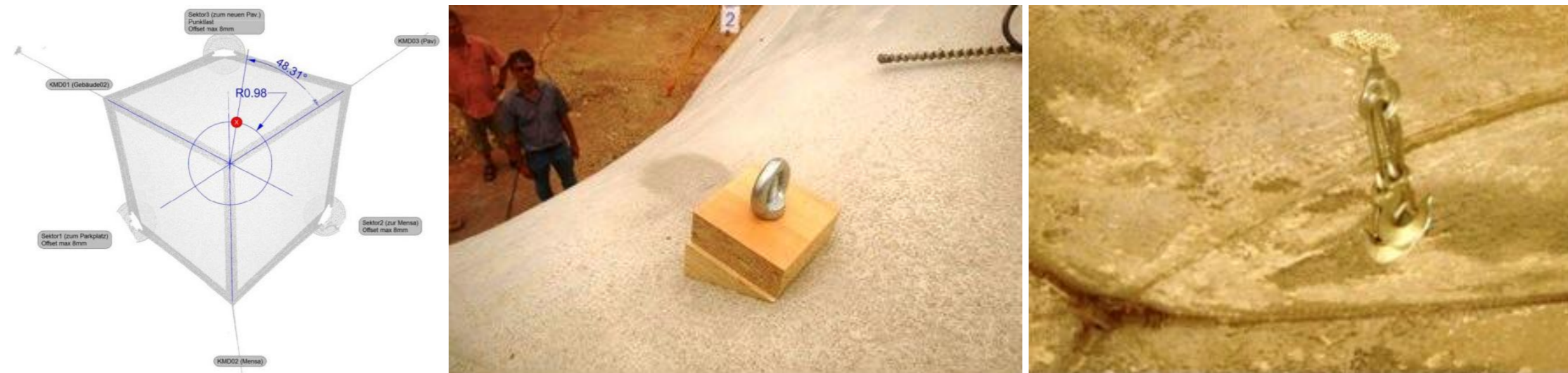
Figure 4.24 – Pictures of 3 rd load test of concentrated load and detail to hung weights from the membrane-concrete shell prototype.
