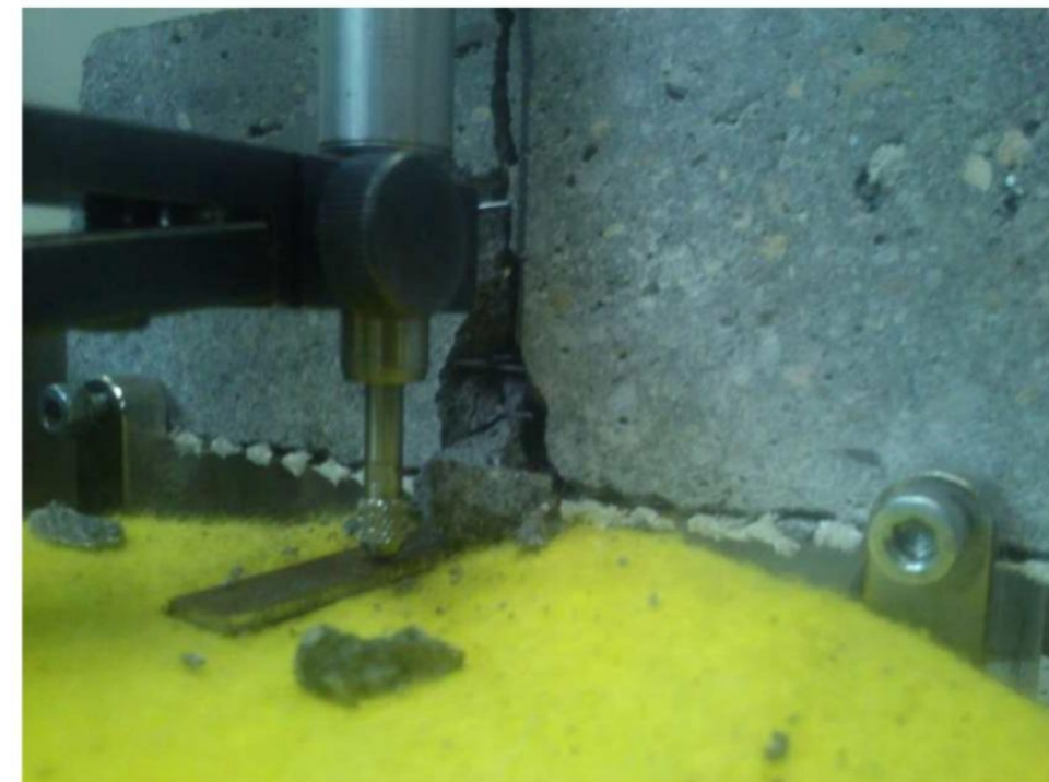
Membrane-Concrete Specimen during testing
