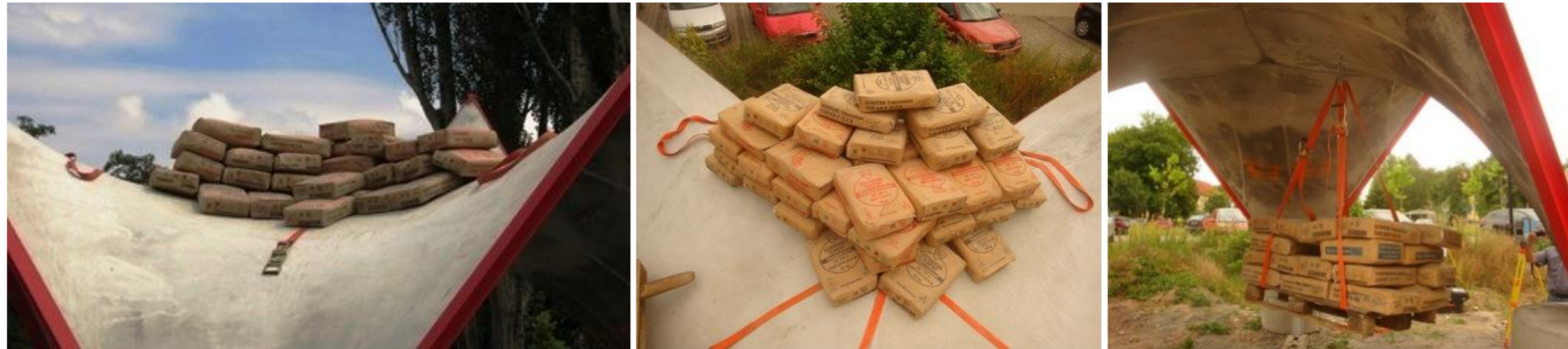
Load Test II-1 – 30 bags ~ 750 kg.
