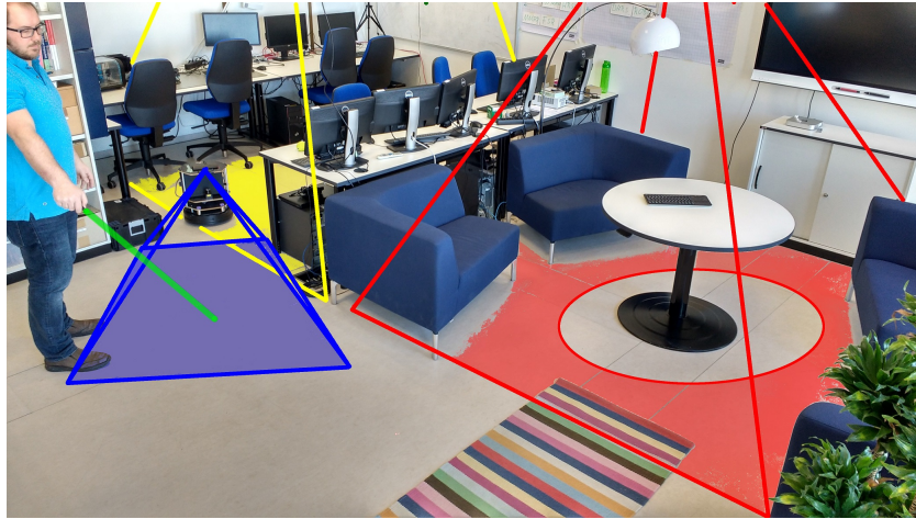
Figure 4.1: A human defines a restriction area in the environment using a laser pointer. The spot is observed by stationary cameras in the environment (yellow and red field of view) and a mobile camera on a robot (blue field of view). A smart display (top right) provides visual feedback of the complex spatial information, and a smart speaker (not shown here) facilitates interaction to switch between different states of the interaction method.
