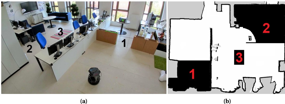
Figure 3.14: (a) Environment with three restriction areas and (b) occupancy grid map of the environment after an interaction process. Numbers are only for visualization purposes.
