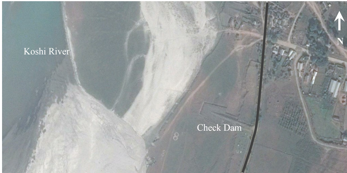
Figure 4.14. Satellite image of the Koshi Riverbank of Chakraghatti showing the check dam and the embankment represented by black line along with part of the flood plain (Google Maps, 2018a).
