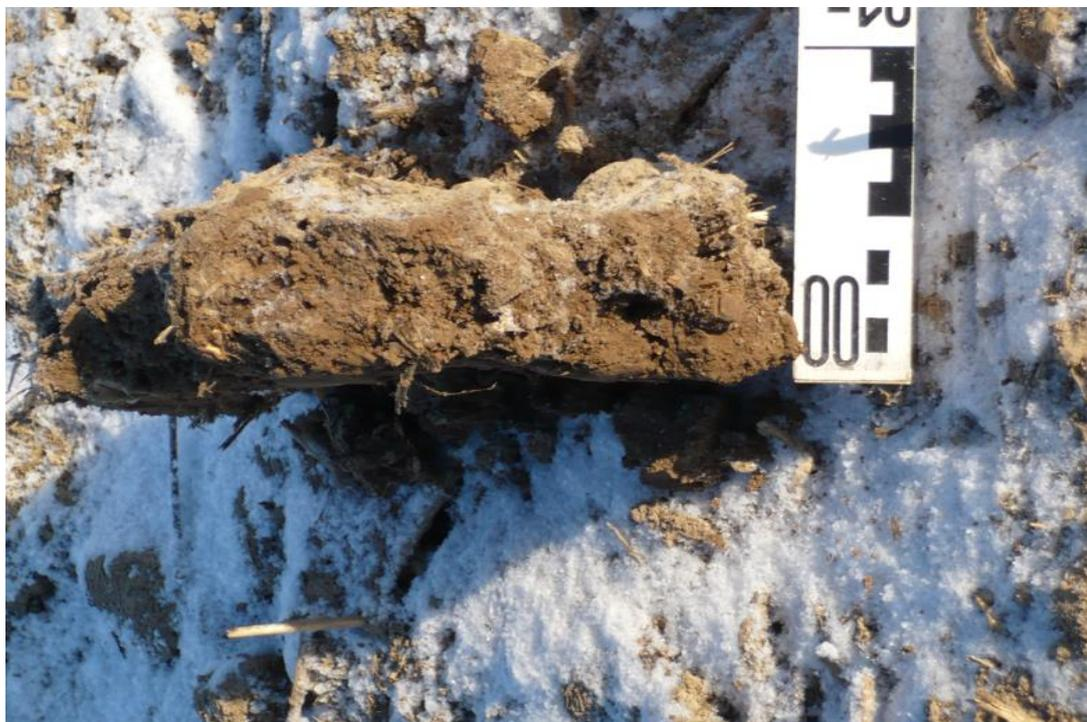
Picture 4.2.1. Determinations of the frost depths by breaking open the frozen layers for each variation at various points and measuring the respective strength.
