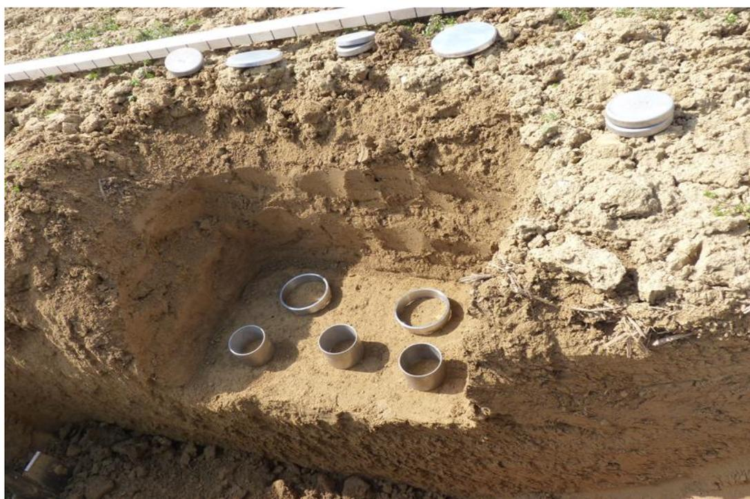
Picture 4.2.2. The physical soil parameters were determined using soil core samplers.
