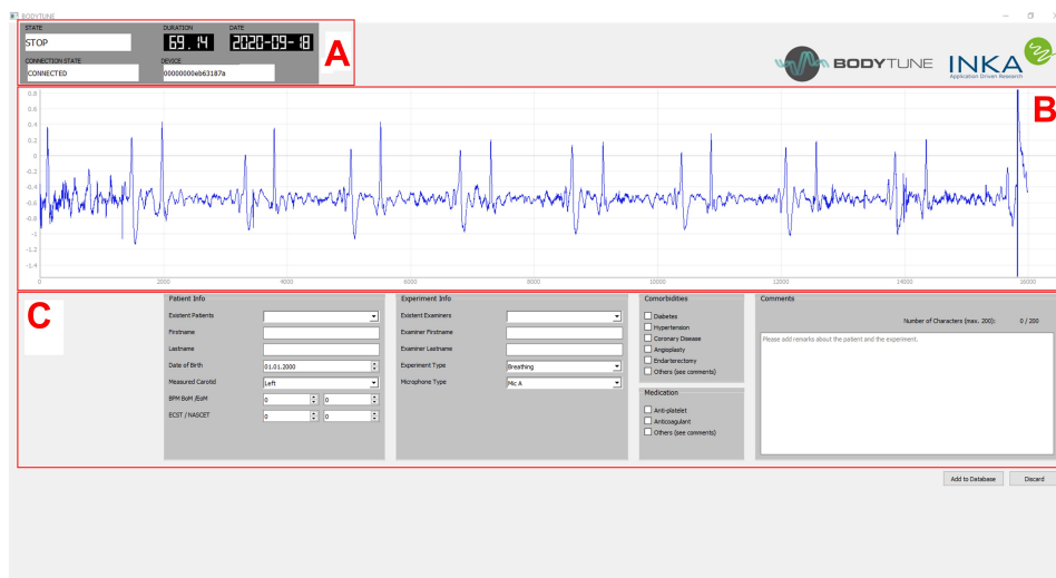
Figure 8 Proprietary desktop application with (A) current state, duration and date of the auscultation, (B) real-time visualization with integrated scaling functionality and (C) input fields for supplementary information regarding patient, experiment and comorbidities or related medication.
