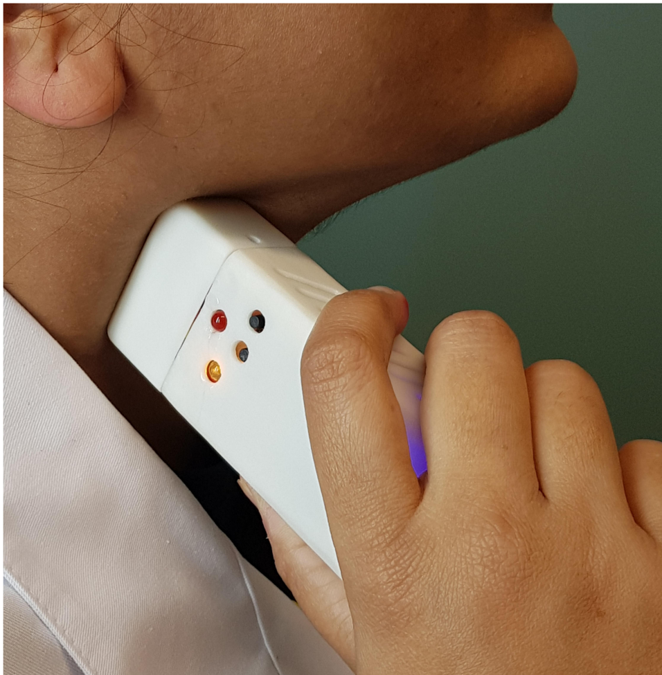
Figure 5 Auscultation of the carotid vascular sound of a voluntary subject with the final CAAS.
