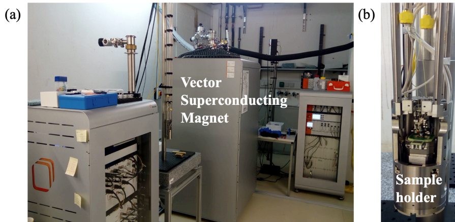
Figure 3.4: MFM setup with model AttoLiquid MFM I from the company Attocube. (a) Chambers for low-temperature measurement and superconducting vector magnet. (b) Sample holder with the magnetic tip and piezo stage.
